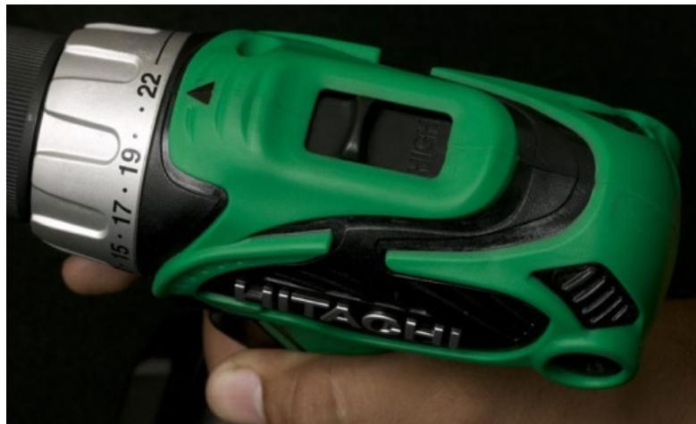
screw, then the clutch starts slipping and you hear a gravelly sound. The clutch should be set to the lightest setting required to just drive the screw to the proper depth and then the clutch will start slipping to prevent stripping the screw head and overdriving the screw too deep. Also, when the screw is fully tightened or if the drill hits an obstruction, the drill jerks to a stop, causing strain on your wrists and hands. Most drill/drivers also have a high or low setting switch on the
